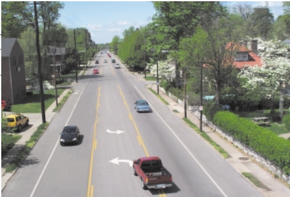
Lexington, Kentucky's "road diet" for Euclid Avenue reduced it from four to three lanes, added bike lanes, made sidewalks safer and the street itself safer and more attractive.
